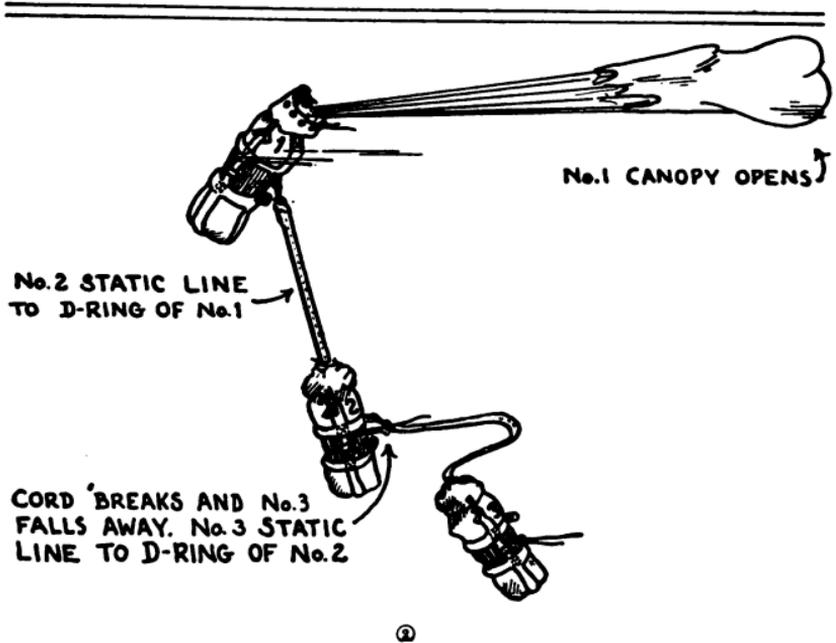
FIGURE 15.—Operation of a "daisy chain."
