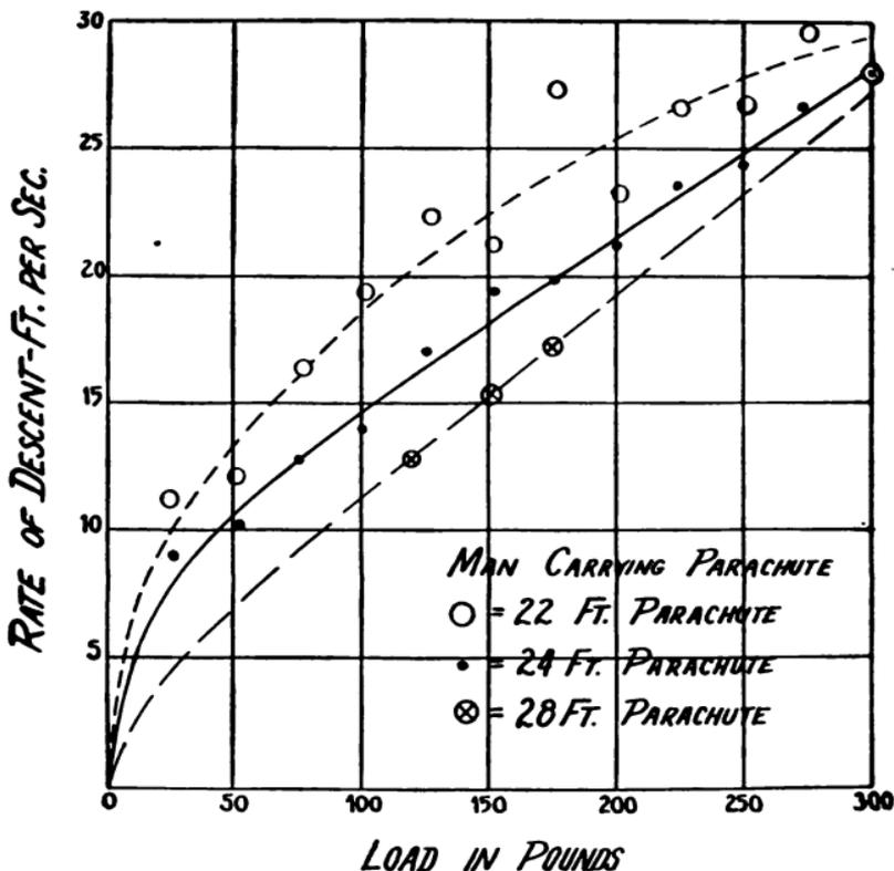
FIGURE 4—Graph showing performance of various sizes of canopies.
