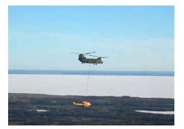
**ABOVE:** The CH-147F Chinook is on its way back to 4 Wing Cold Lake with the Griffon securely slung below it.
