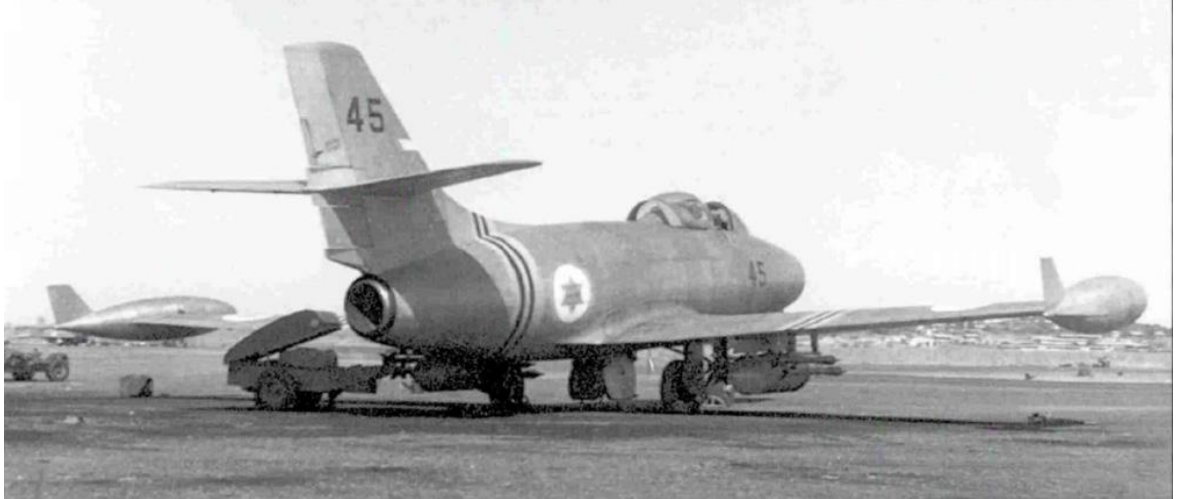
Ouragan armed with eight HVAR rockets and a pair of napalm canisters under its wings. Note the yellow and black identification bands on the wings and rear fuselage.
